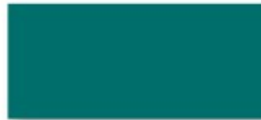
Sanodye Blue 2LW 0.4 g/l Sanodure Fast Gold L 0.2 g/l
